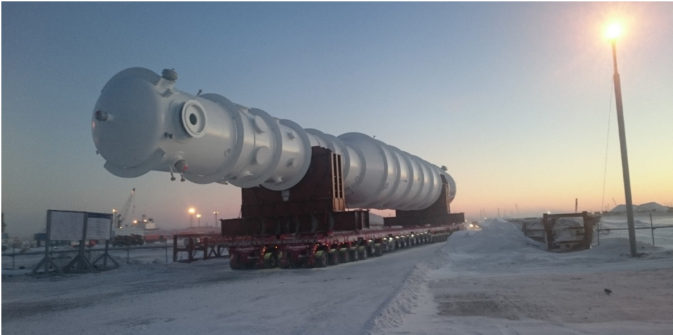
Figure 5. An MCHE being moved to the field site in the Arctic Circle.
